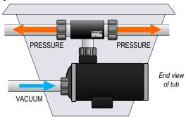
In-Line Heaters are to be installed as shown:
