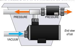
In-Line "Pump Suction Side" Heaters are to be installed as shown:
